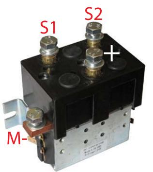
Labels correspond to Alltrax wiring diagrams. Note that the M- buss bar runs all the way through the contactor. So sometimes it will be on the opposite side and it makes no difference.
